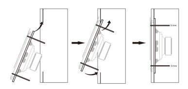
Remove the speaker grill . With access to the four screws holding the speaker to the mounting bracket loosen them as needed to allow space for the drywall. Next, with the terminals at the bottom of the speaker, slide the top part of the mounting bracket into the opening and up behind the drywall. (**See Diagram 3**) Then slide the bottom of the metal bracket into the opening. The speaker will be flush against the wall.
